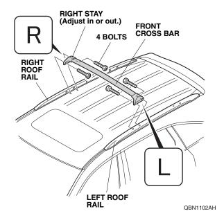
3. Install the rear cross bar to the left roof rail and right roof rail with four bolts. Torque the bolts to 10 N·m (7.4 lbf·ft).
